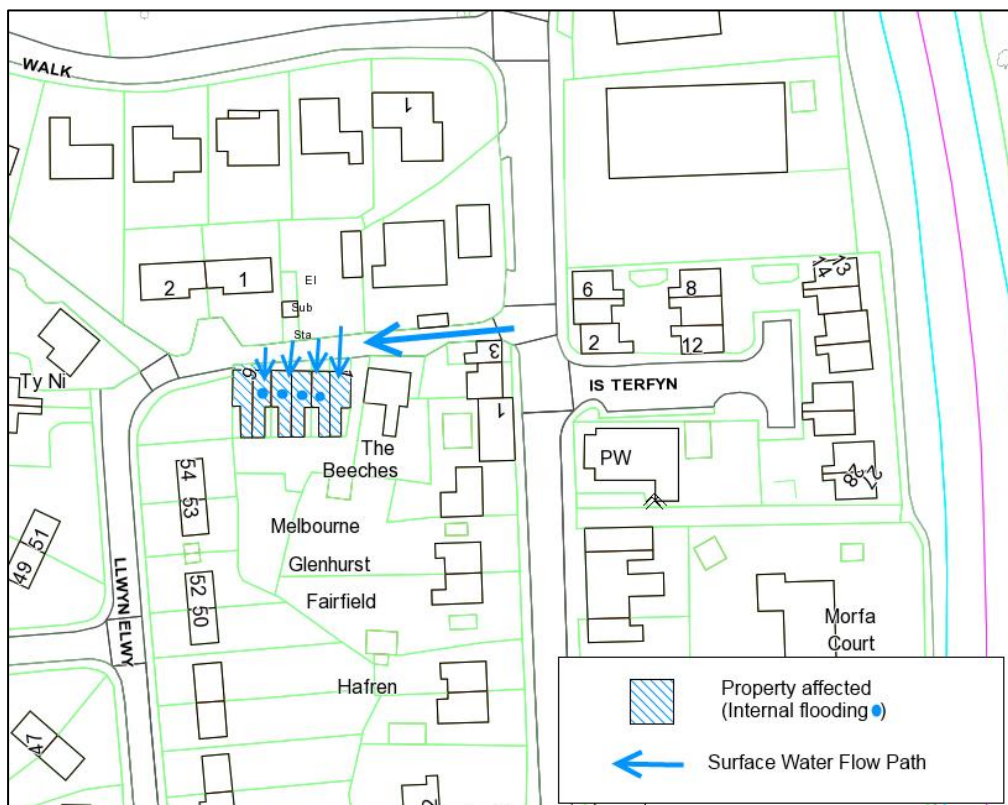
Figure 16 - Low lying properties suffered internal flooding via front doors, other properties flooded due to private drainage systems failing.
