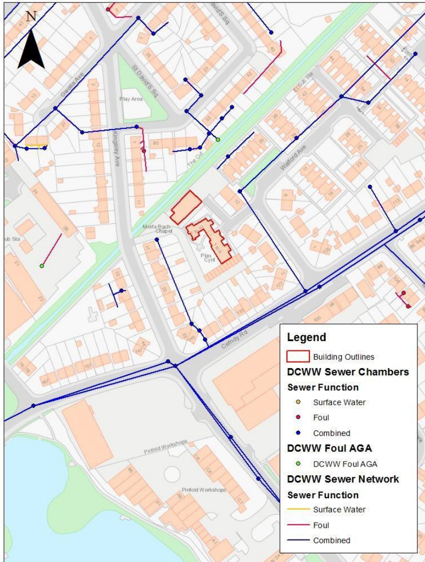
Figure 20: Welsh Water Piped System
