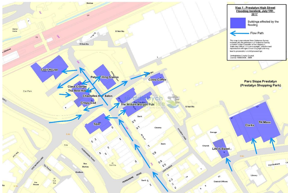
Figure 9 – Lower Prestatyn High Street and Shopping Park – Properties Flooded
